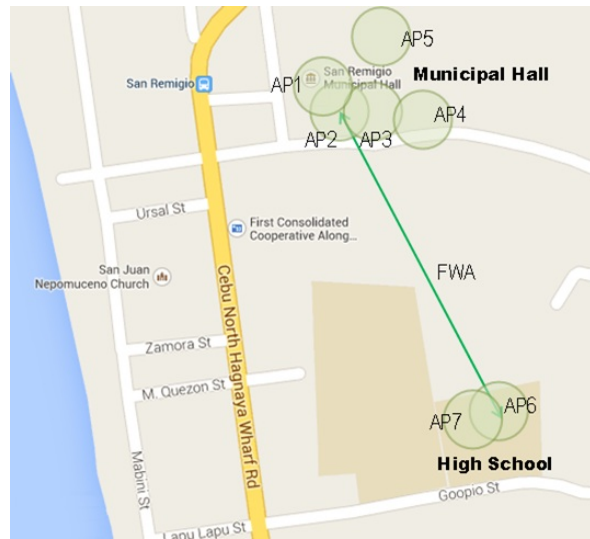
<Locations of Wi-Fi access points and FWA equipment>
